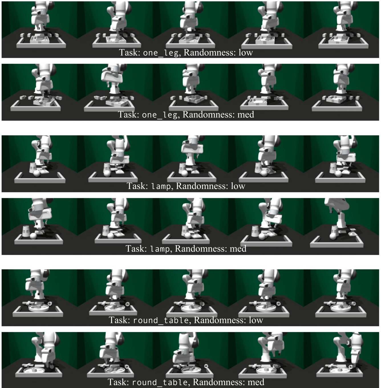
Fig. 17. Examples of initial scene layouts for the tasks from the FurnitureBench task suite [5], one_leg, lamp, and round_table, with different levels of initial part pose and obstacle fixture randomness.
